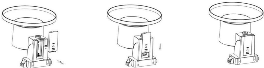
Figure 16: Rain gauge sensor battery installation diagram
